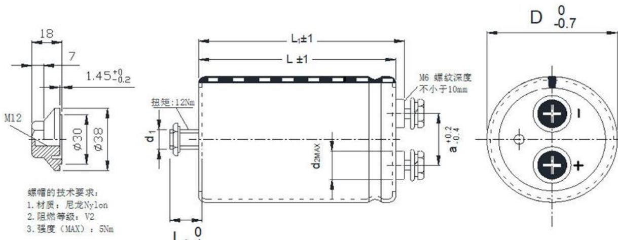
D: 76.9      d<sub>2MAX</sub>: 17.4      L: 155      L<sub>1</sub>: 160.8      螺丝: M6X12不配送
